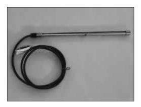
The design of the ionizing bar EI Ex T complies with the European ATEX directives. In combination with power pack EN 92 Ex or Multistat Ex, it is suitable for use in manufacturing locations with potentially explosive atmospheres resulting from gases of explosion group IIA, temperature classes T4 to T6.
