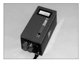
The Multistat Ex is a modern high-voltage power pack with fully electronic watchdog function. It is fitted with an automatic fault alarm, an analog display for high-voltage monitoring and an output jack for the connection of peripheral alarm units. This power pack must always be installed outside the potentially explosive atmosphere. It is approved for the operation of ionizing bar EI EX T and ring ionizers RI Ex O/M/V.
